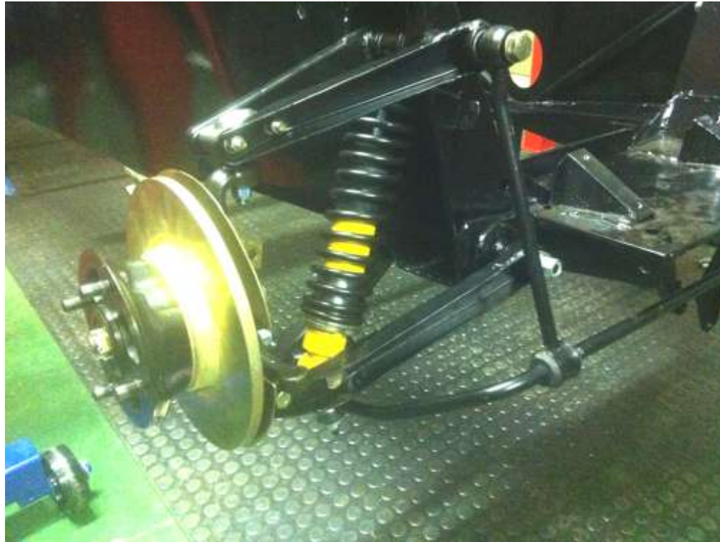
Front suspension after power coating, electro plated discs, new hub bearings, vertical links, trunnion, bushes and dampers.
