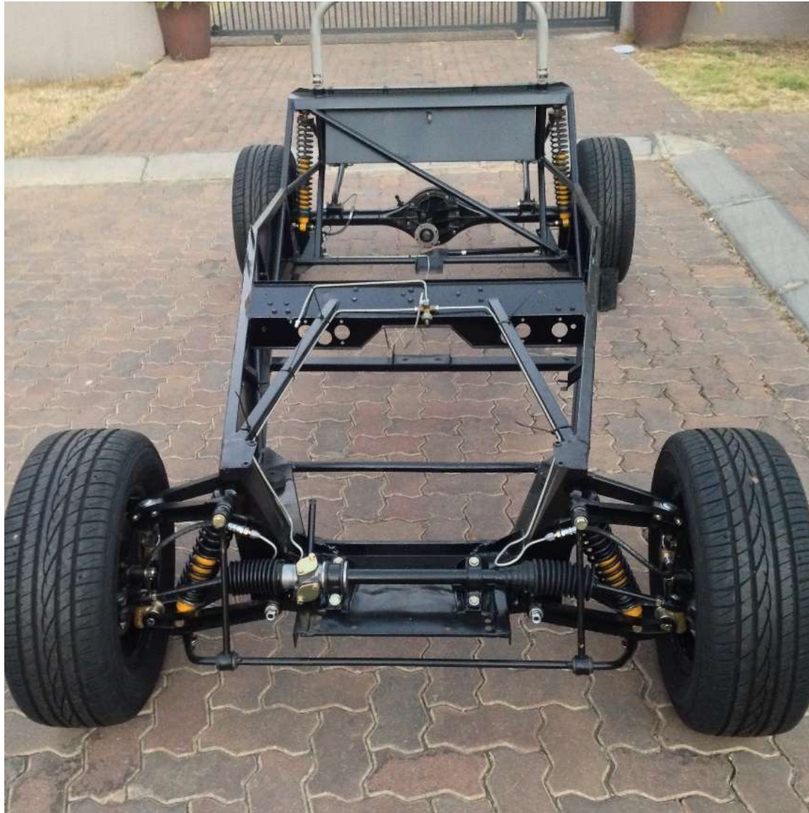
Restored chassis and brake lines
